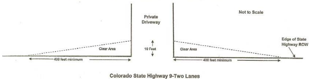
Figure 2 Example of "Sight Distance Triangle" Based upon AASHTO State Guidelines used by CDOT for Driveway Access
