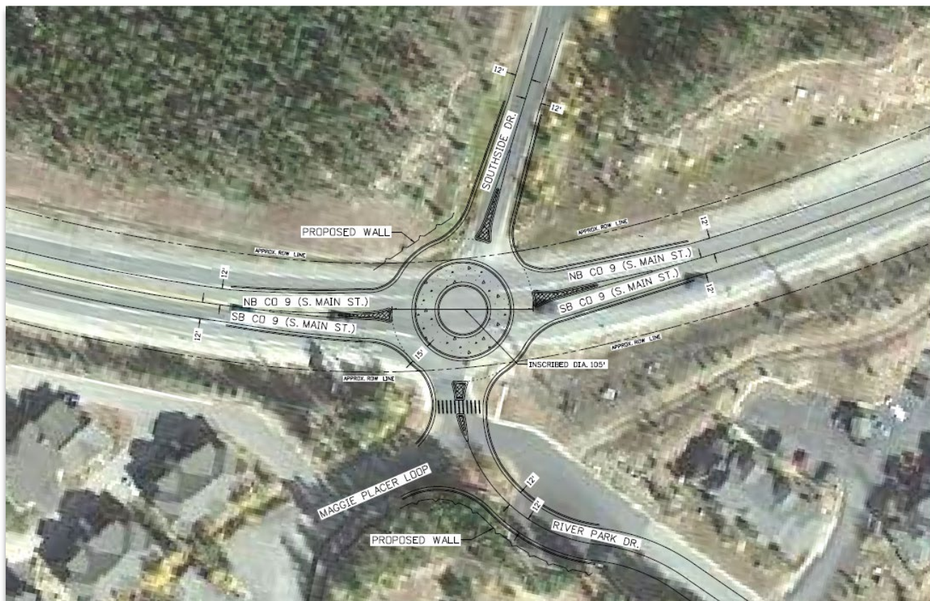
Figure 9-5. Conceptual Roundabout Design – CO-9 and Southside Drive/River Park Drive
