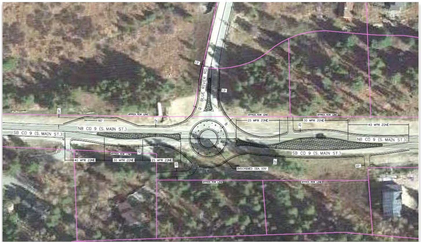
Figure 9-6. Conceptual Roundabout Design – CO-9 and Blue River Road
