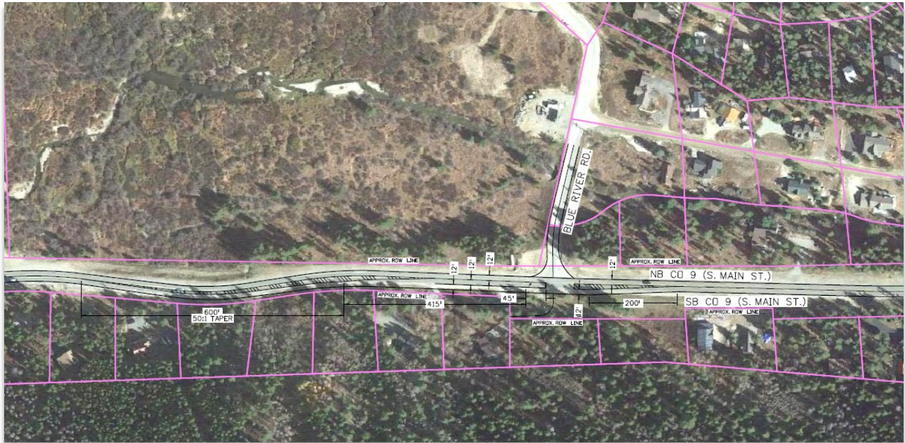
Figure 9-7. Conceptual Intersection Design – CO-9 and Blue River Road
